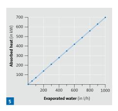
absorption of the microscopic, atomised water droplets in the air causes heat to be drawn out of the room. The principle of adiabatic evaporative cooling achieves an extremely cost-effective lowering of the room temperature: 100 l water from a high-pressure humidification system absorbs around 70 kW heat while consuming only 0.6 kW of energy, achieving a potential reduction in room temperature of between 2 °C and 5 °C.
