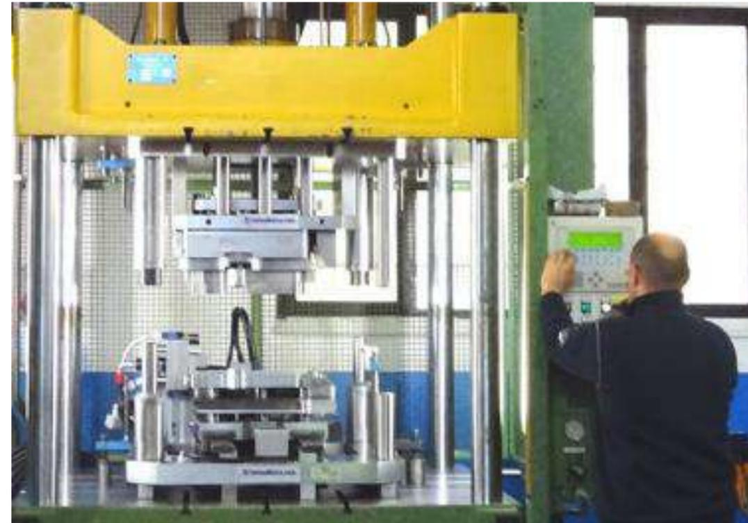
Testing with in house trimming press
