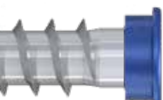
Stepped head • Raised wood fibres are separated by the lower step and remaining material is covered by the upper disc • Clean fitting appearance
