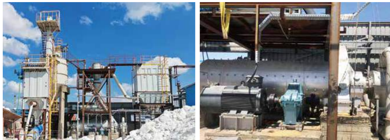
1T/H Talc Ball Mill Grinding Production Line In Egypt, Year 2026 (Φ1.5*4.5m Ball Mill)
