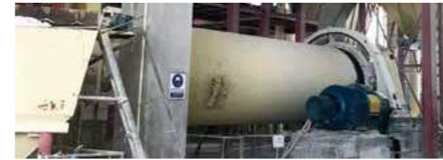
50,000tons/Year Silica and Feldspar Ball Mill Plant In Egypt, Year 2013 ( \Phi 2.2 \times 7.5\text{m} Ball Mill)
