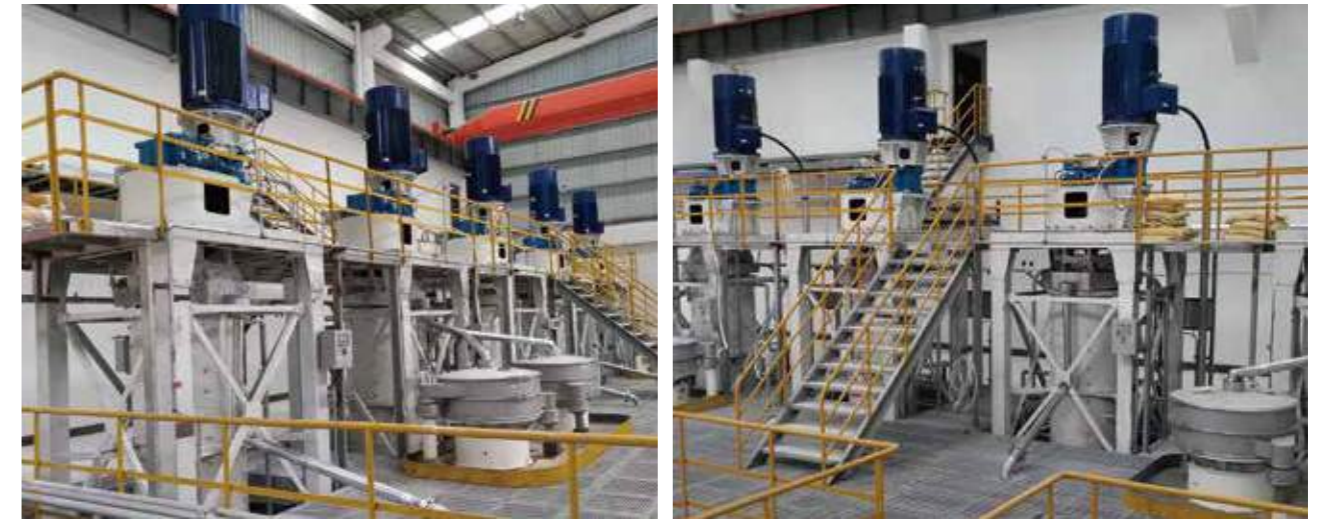
Wet Grinding Mill VMG3600 for Paper industry in China, year 2016
