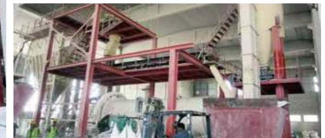
50,000tons/Year Silica and Feldspar Ball Mill Plant In Egypt, Year 2013 ( \Phi 2.2 \times 7.5\text{m} Ball Mill)
