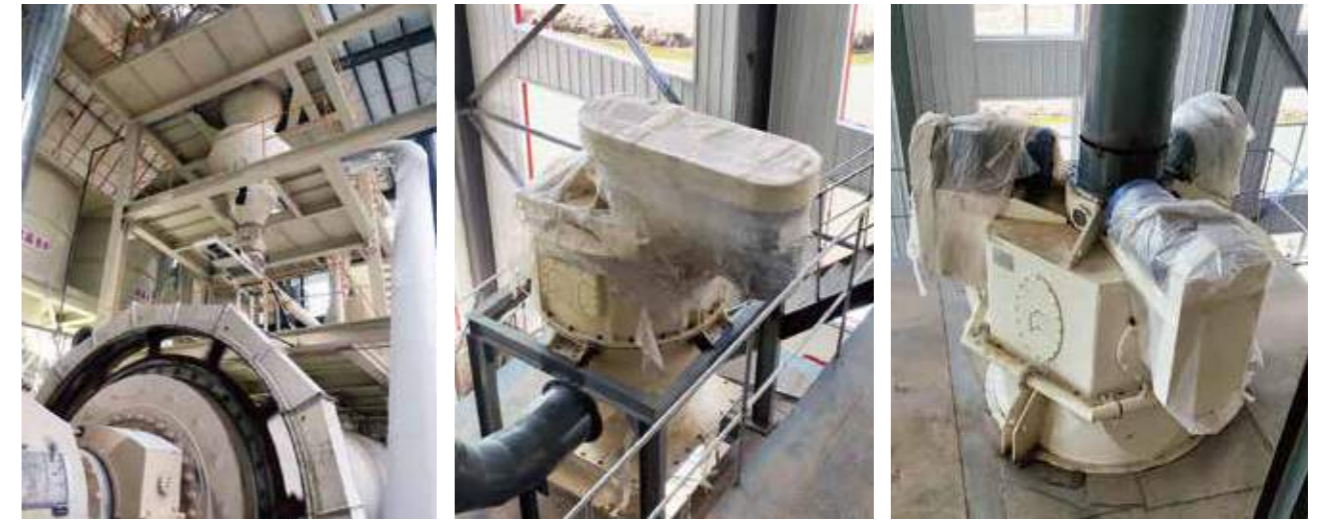
35,000tons/Year Brucite ball mill plant in China, year 2021 ( \Phi 2.6 \times 9.0 m Ball Mill)
