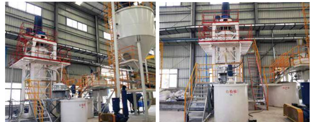
Wet Grinding Mill VMG3600 for nano-CaCO3 in China, year 2021
