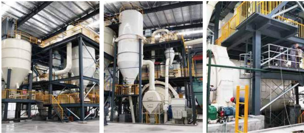
30,000tons/Year Zirconium Dioxide ball mill plant in China, year 2024 (Φ2.4*8.0m Ball Mill)
