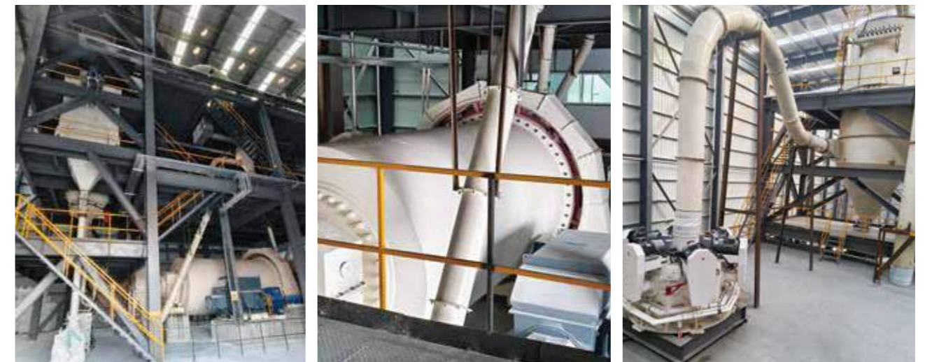
20,000tons/Year Ultrafine quartz ball mill plant in China, year 2020 ( \Phi 3.2 \times 5.7 m Ball Mill)
