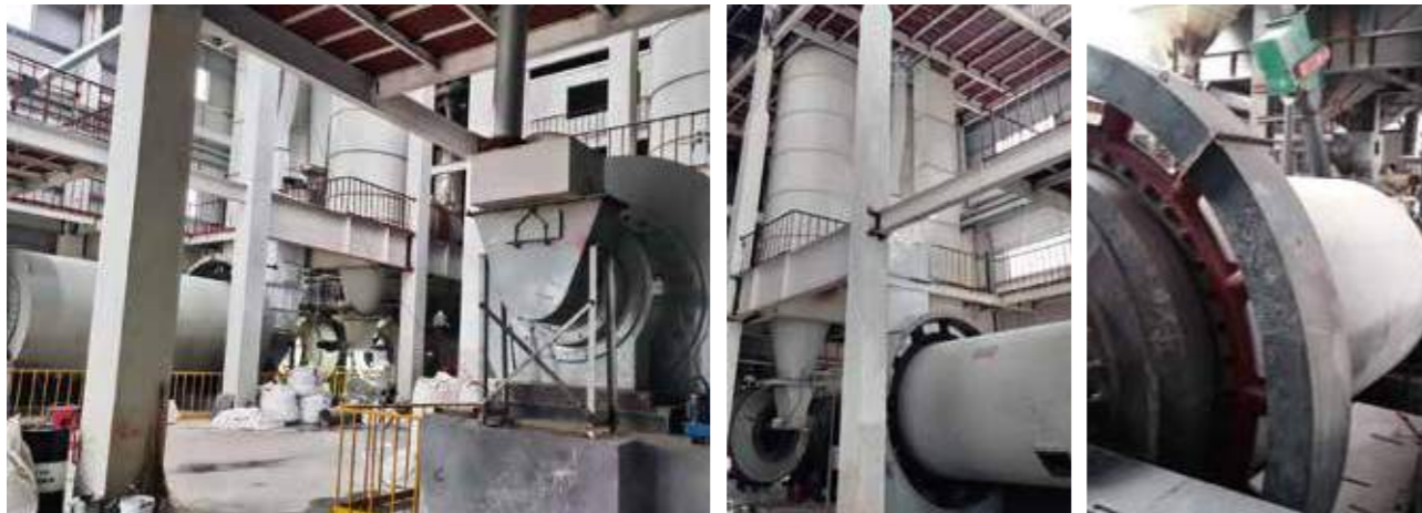
40,000tons/Year Aluminium Oxide ball mill plant in China, year 2020 ( \Phi 2.4 \times 8.0 m Ball Mill)
