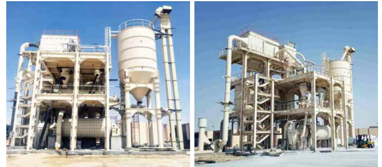
20,000tons/Year Ultrafine quartz ball mill plant in China, year 2020 (Φ3.2*5.7m Ball Mill)
