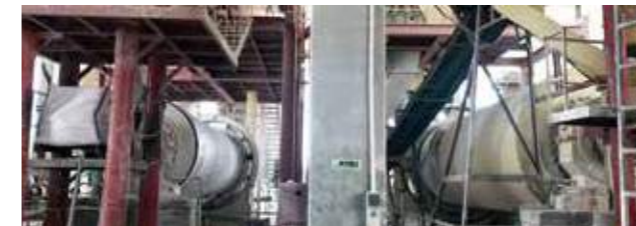
120,000tons/Year Silica and Feldspar Ball Mill Plant In Egypt, Year 2014 (2sets Of \Phi 2.4 \times 8.0\text{m} Ball Mill)
