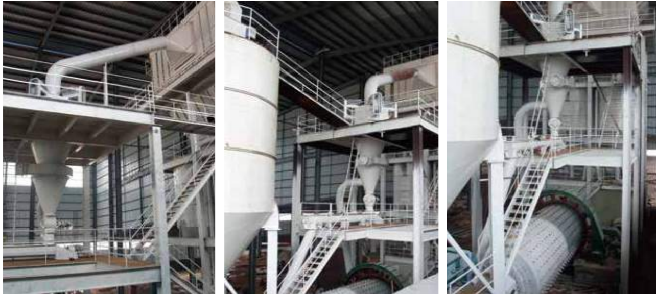
30,000tons/Year Dolomite ball mill plant in China, year 2009 ( \Phi 2.4 \times 8.0 m Ball Mill)
