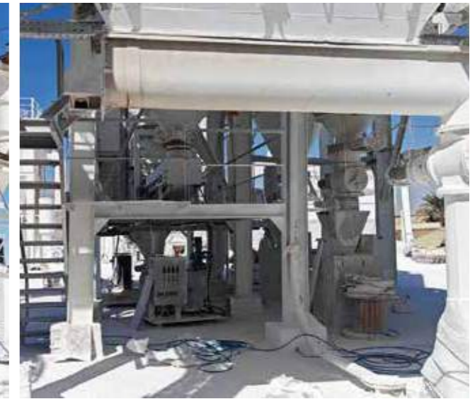
40,000tons/Year Calcium Carbonate Ball Mill Plant and Coating Plant In Egypt, Year 2025 ( \Phi 2.2 \times 5.5\text{m} Ball Mill)
