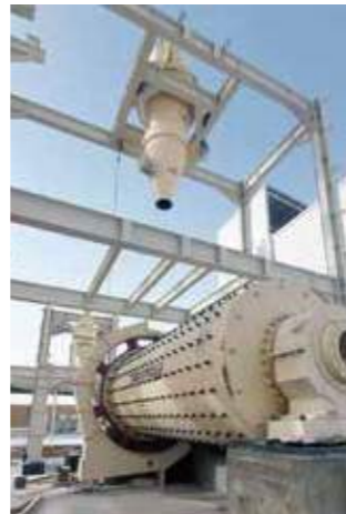
40,000tons/Year Calcium Carbonate Ball Mill Plant and Coating Plant In Egypt, Year 2023 ( \Phi 2.2 \times 5.5\text{m} Ball Mill)
