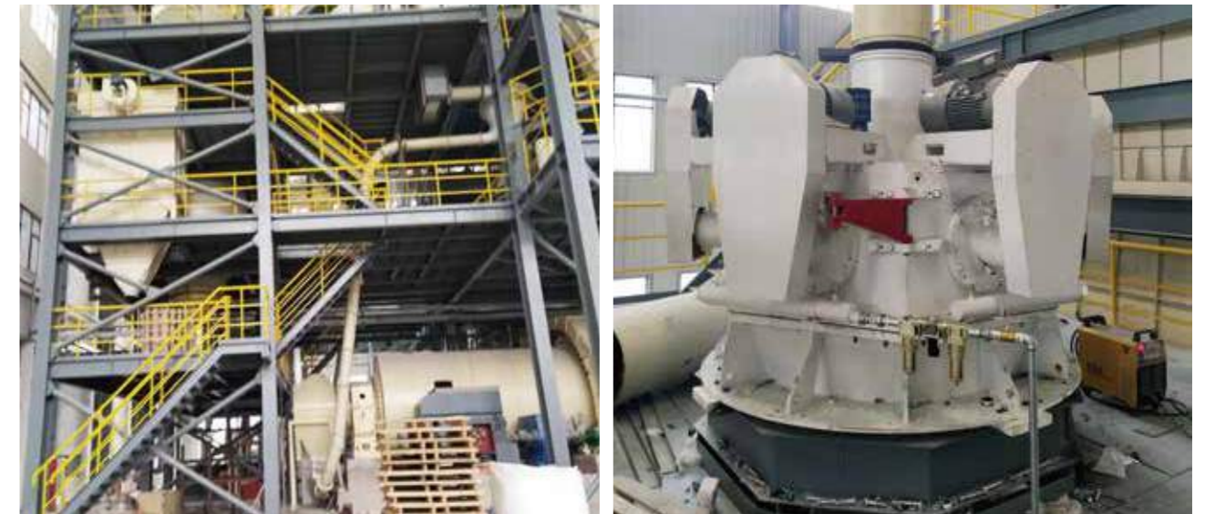
10,000tons/Year quartz ball mill plant in China, year 2022 ( \Phi 2.4 \times 8.0 m Ball Mill)
