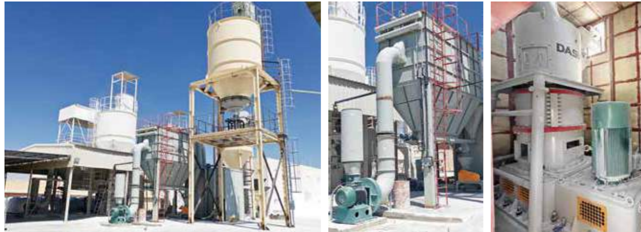
3T/H DR-28 Ring Roller Mill Calcium Carbonate Processing Plant In Minya, Egypt, Year 2026
