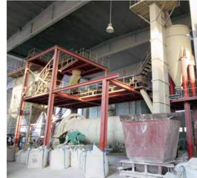
50,000tons/Year Silica and Feldspar Ball Mill Plant In Egypt, Year 2013 ( \Phi 2.2 \times 7.5\text{m} Ball Mill)
