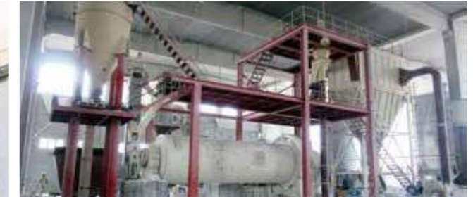
40,000tons/Year Calcium Carbonate Ball Mill Plant and Coating Plant In Egypt, Year 2025 ( \Phi 2.2 \times 5.5\text{m} Ball Mill)
