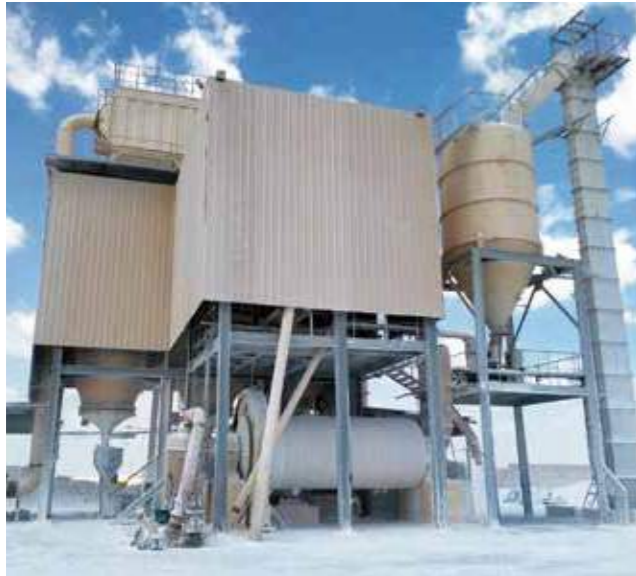
Calcium Carbonate Ball Mill Plant In Egypt, Year 2021 ( \Phi 2.2 \times 5.5\text{m} Ball Mill)
