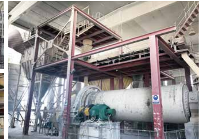
120,000tons/Year Silica and Feldspar Ball Mill Plant In Egypt, Year 2014 (2sets Of \Phi 2.4 \times 8.0\text{m} Ball Mill)
