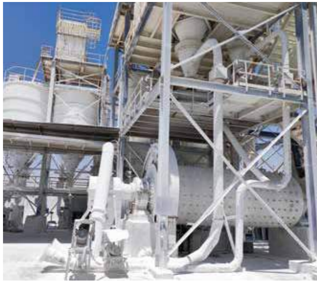
60,000tons/Year Calcium Carbonate Ball Mill Plant In Egypt, Year 2021 ( \Phi 2.4 \times 6.0\text{m} Ball Mill)
