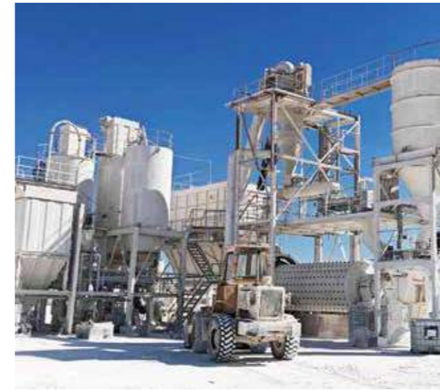
40,000tons/Year Calcium Carbonate Ball Mill Plant and Coating Plant In Egypt, Year 2025 ( \Phi 2.2 \times 5.5\text{m} Ball Mill)
