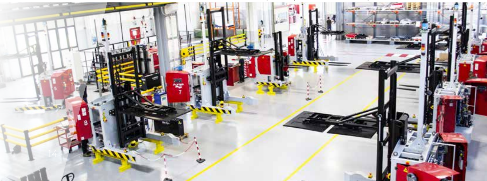
Part of the OCME production plant dedicated to the assembly and test area for LGV vehicles
