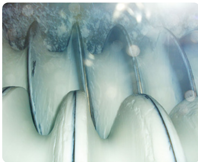
Product coating on screw flights
