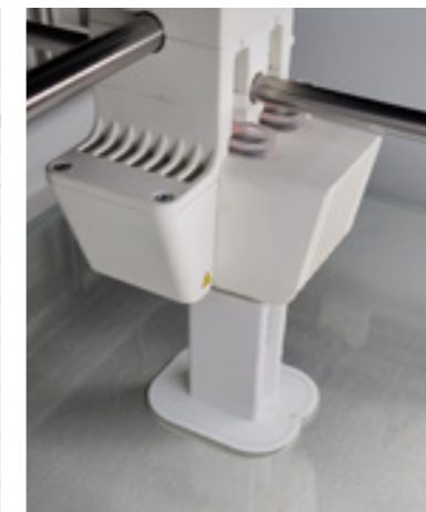
Printing of samples by the Fused Deposition Modeling (FDM) technique
