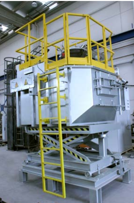
Ladder and security barrier
