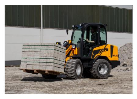
**Caption:** The new Schäffer 2430-2 is set to become a firm favourite thanks to its efficient drive concept and its high lifting capacity; in use here with maximum ballast.
