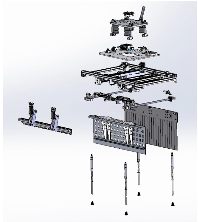
Figure 2 Exploded view of a gripper configuration with clamping plate
