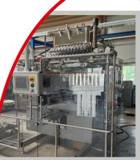
The market is constantly demanding more products with recyclable or compostable film. GKS packaging machines can basically pack all liquids in these films, with minor adjustment of the temperature and sealing pressure parameters. Pressure tests at 2 bar and endurance tests lasting 9 months were carried out in customer laboratories and successfully completed.
