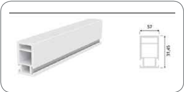
ADAPTER PROFILE WITH INSULATION
