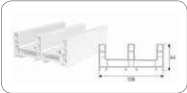
THREE TRACK SLIDING FRAME PROFILE
