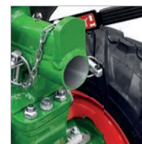
Additional fixture for towed attachments e.g. ploughs
