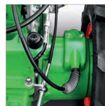
Robust steering brake clutch for easy steering
