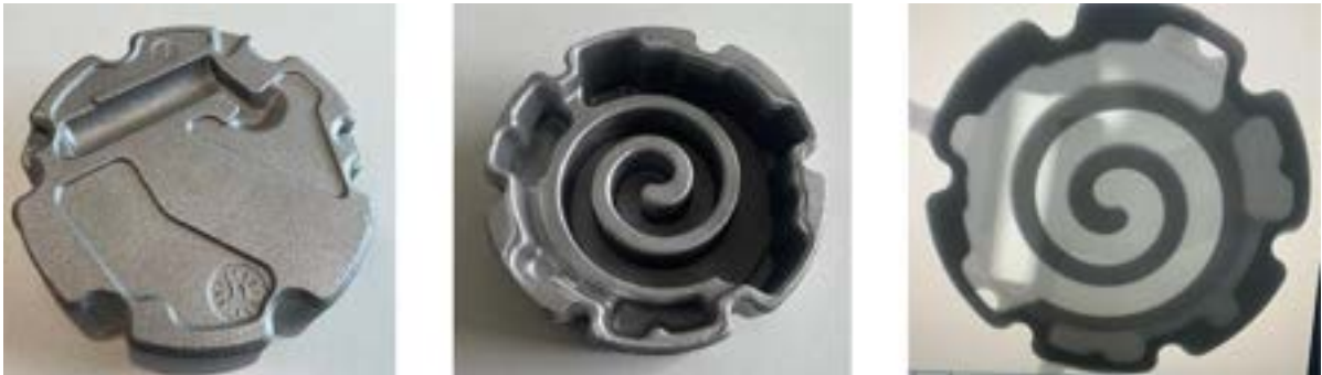
Absence of porosity or inclusions. Thickness reduced to 2.5 mm.
