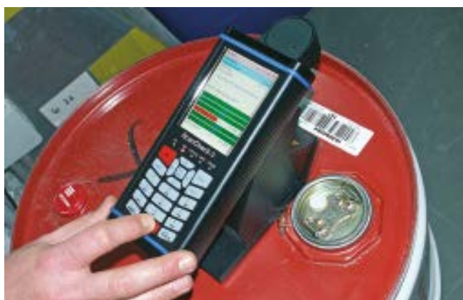
Verification of barcodes on metal drums
