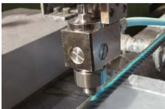
Color marking of wire cables
