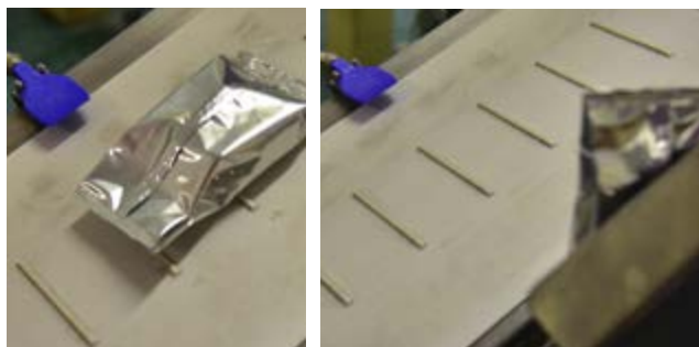
Defective packages are automatically sorted out by a reject unit.
