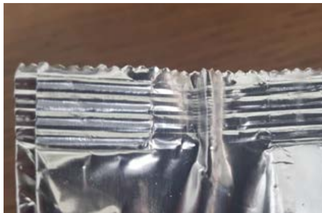
Package with undesired plies ejected by SealScope ® system
