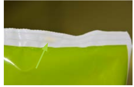
Cheese parts in the seal in a bag rejected by SealScope®
