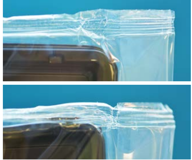
Defective packages rejected by the SealScope ® system with folds (top) and plastic tray in seal (bottom).
