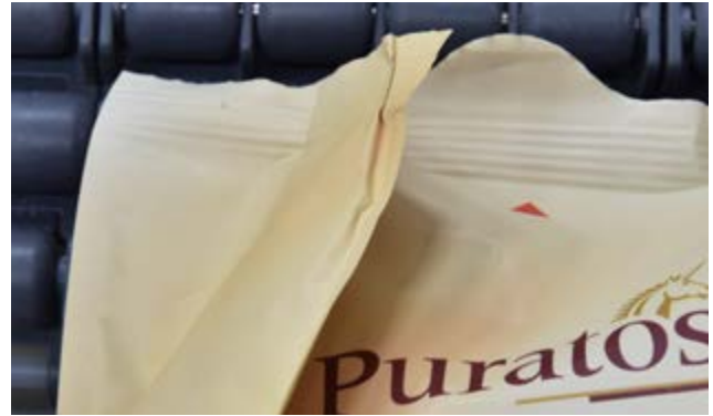
Rejected package due to fold in the seal.
