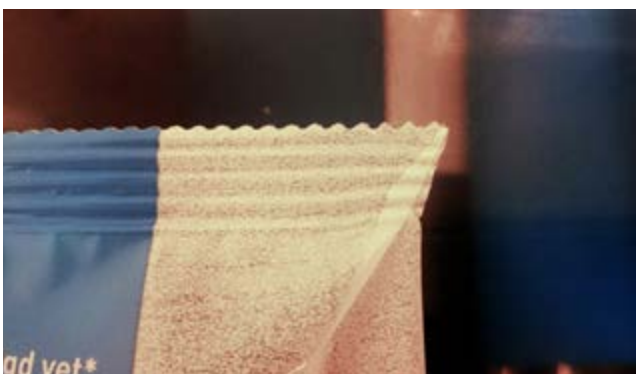
Wrinkles in the seal can lead to leaks in the cheese package
