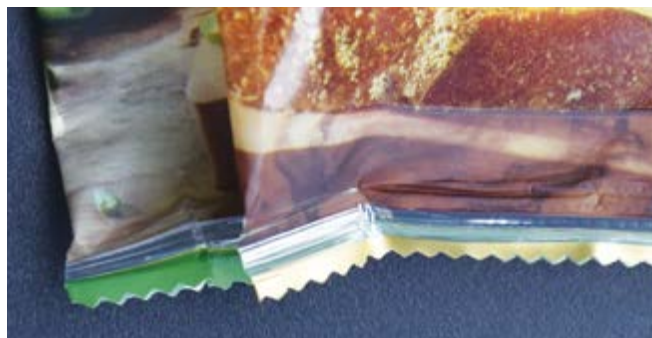
Rejected package with folds in the seal.
