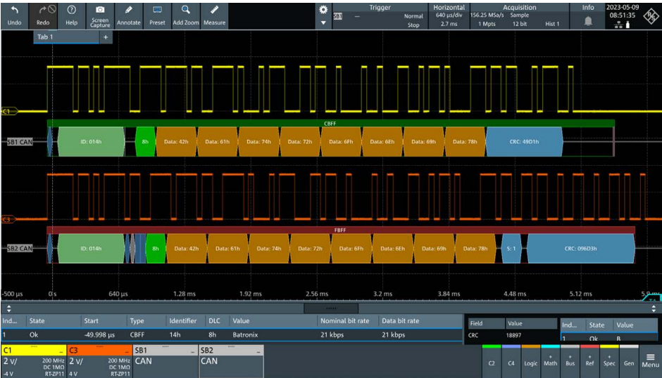
Screenshot: CAN interface decoding and decoder table
