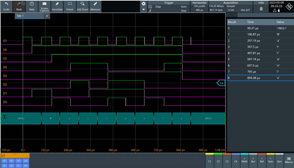
Screenshot: Parallel bus interface decoding and decoder table
