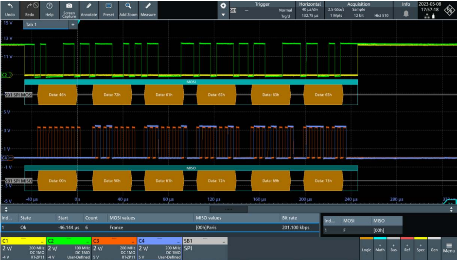
Screenshot: SPI interface decoding and decoder table
