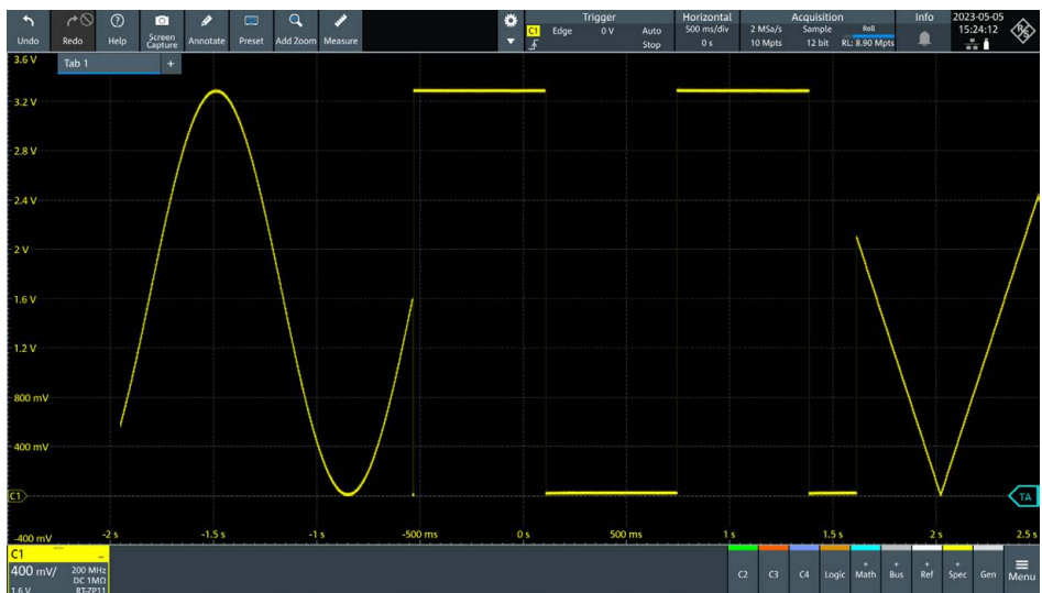
Screenshot: Roll mode with changing signal curves, achieved by switching Select 1 during measurement
