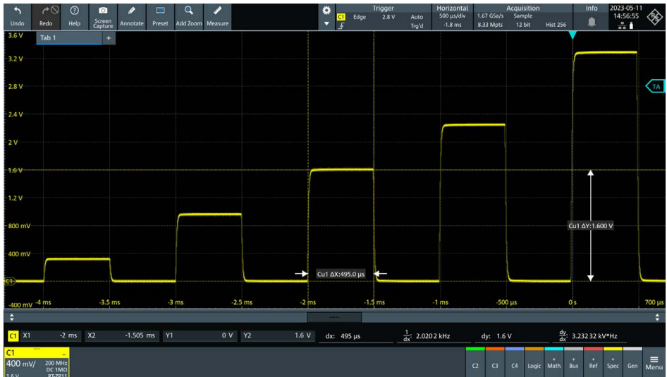
Screenshot: Measuring a pulse with the cursor function
