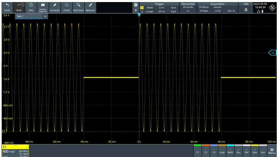
Screenshot: Triggering with the pulse width trigger on a burst
