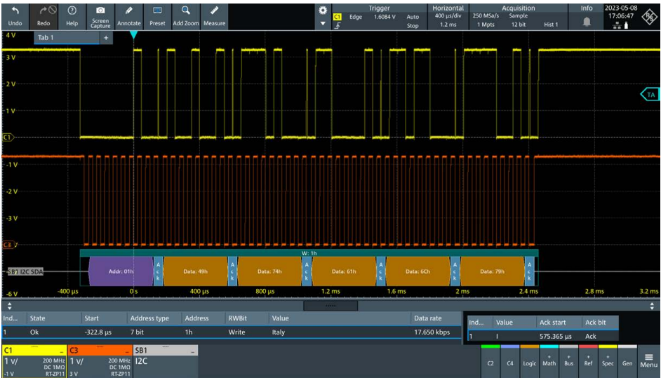
Screenshot: I 2 C interface decoding and decoder table
