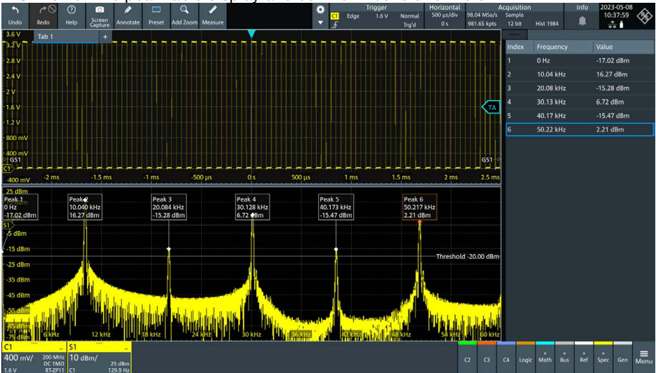
Screenshot: FFT analysis of a square wave signal with clearly visible harmonics
