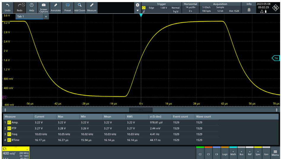
Screenshot: Automatic measurement of various signal parameters
