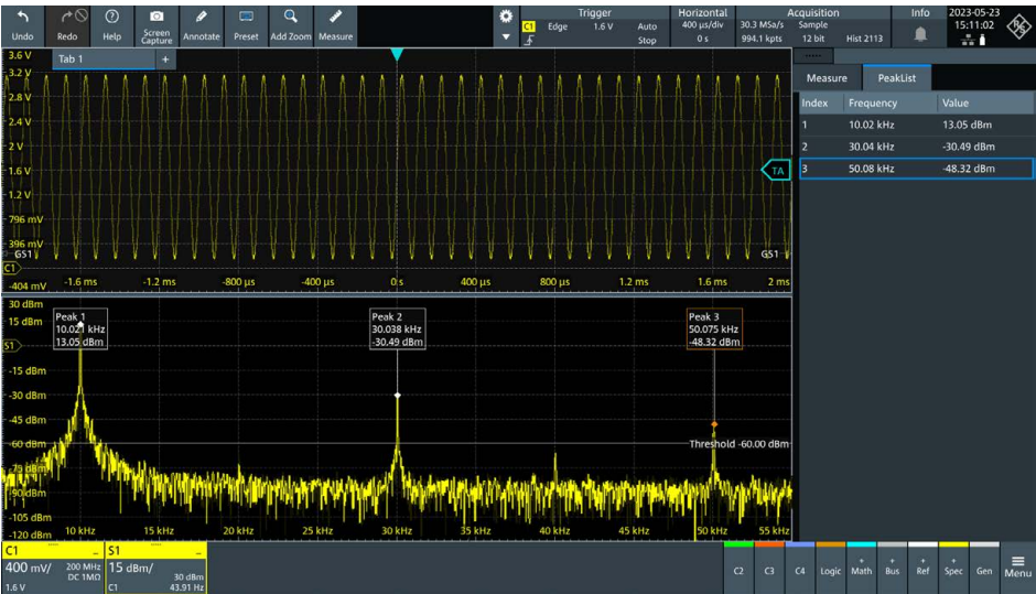
Screenshot: FFT analysis of a sinusoidal signal with clear peaks at 30 kHz and 50 kHz (HD3, HD5)
