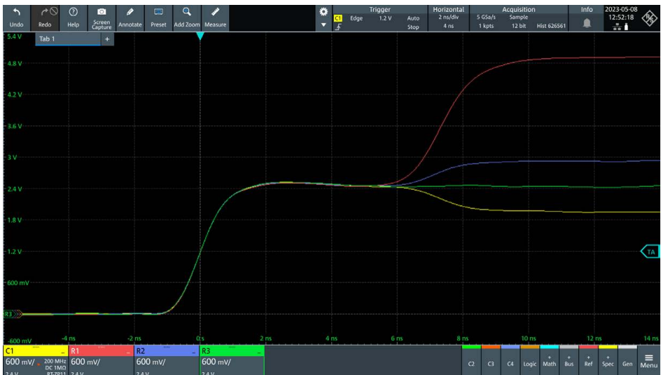
Screenshot: The effect of correct termination for “electrically long” signals
