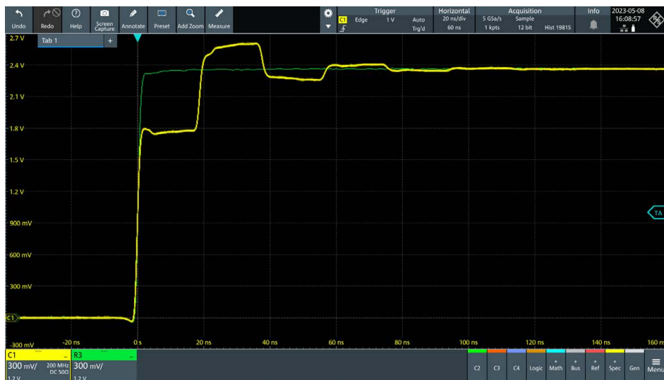
Screenshot: Reflections on non-terminated lines
