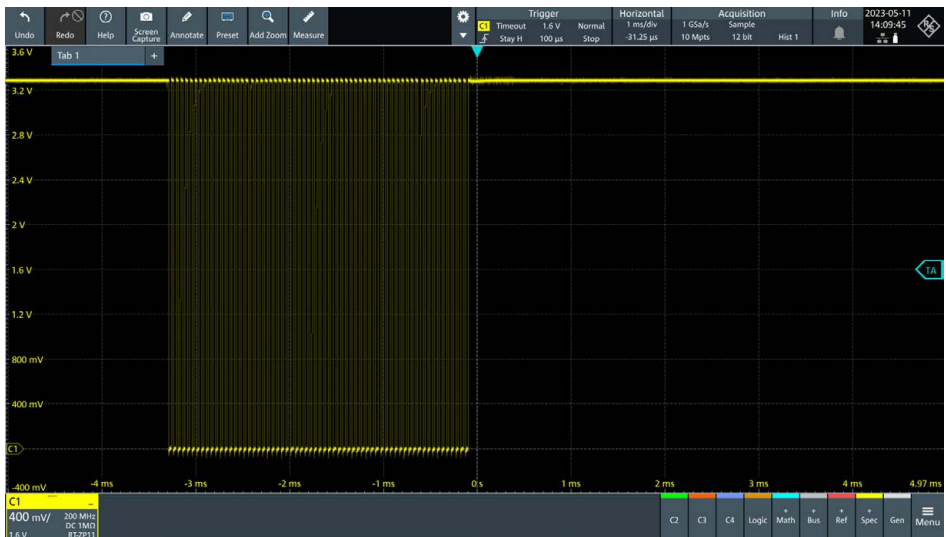
Screenshot: Triggering with the dropout or timeout trigger on the end of a data transmission
