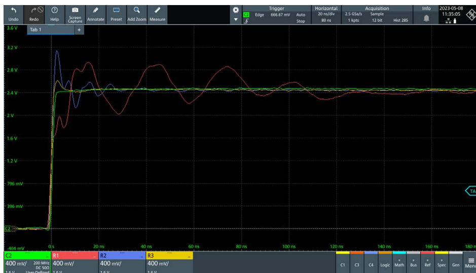
Screenshot: The effect of different probe ground connections at fast edges
