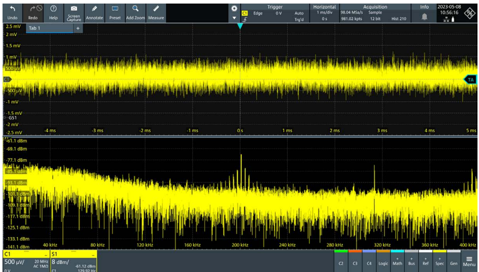
Screenshot: FFT noise analysis of a DC voltage from the function generator of the demo board
