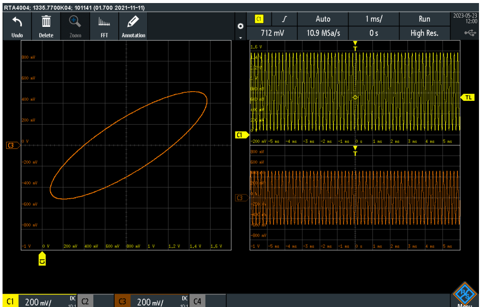
Screenshot: XY diagram of two signals
