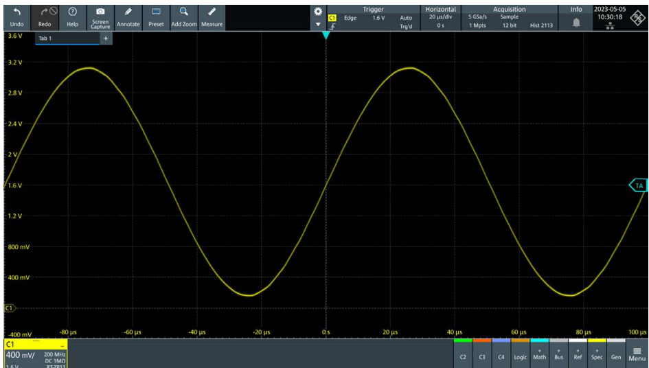
Screenshot: A 10 kHz sinus signal, scaled to fit the screen
