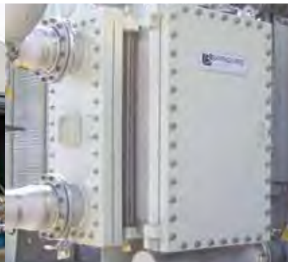
Platulaire® type X 4 doors on white liquor in pulp & paper
