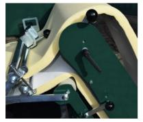
New sponge belt technology with a new foam type for the absorption of sand grains of max. 4mm. The sponge belt is fed on a conveyor belt avoiding its expansion and side wards running, so that a
