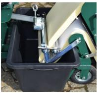
65 litres water container provides a very large time frame between the exchange of water.
