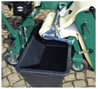
The squeezing unit is flipped up allowing the simple and easy exchange of the water container.
