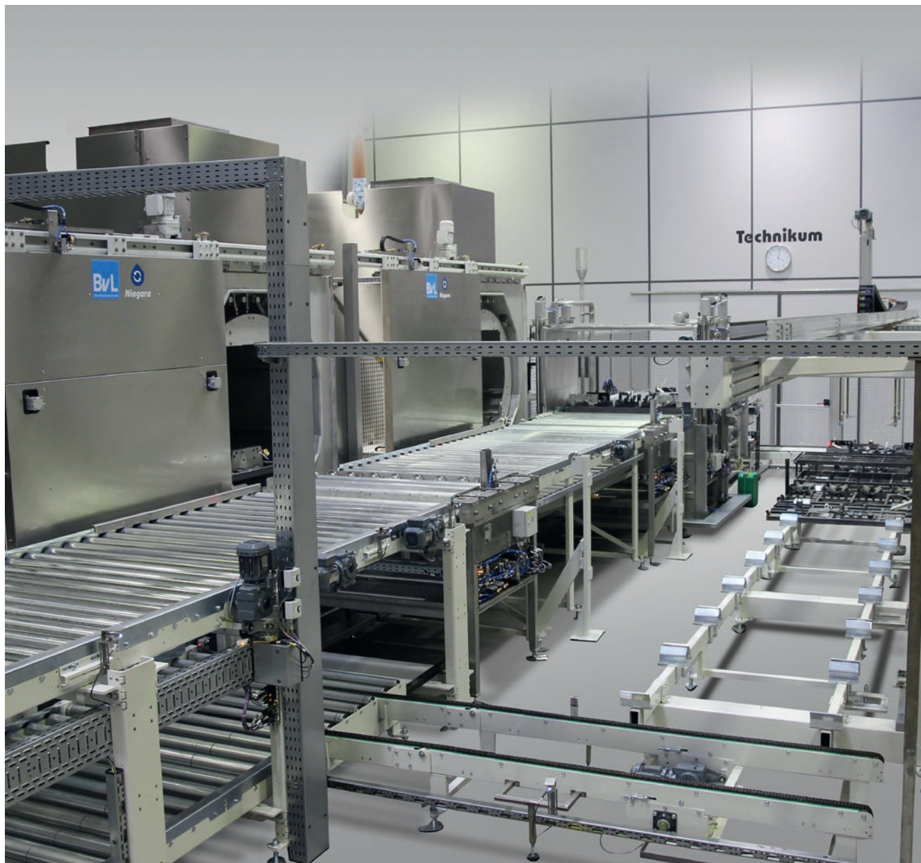
NiagaraDFS as double system with Nevada drying, roller conveyor, bridge loader and workpiece carrier station
