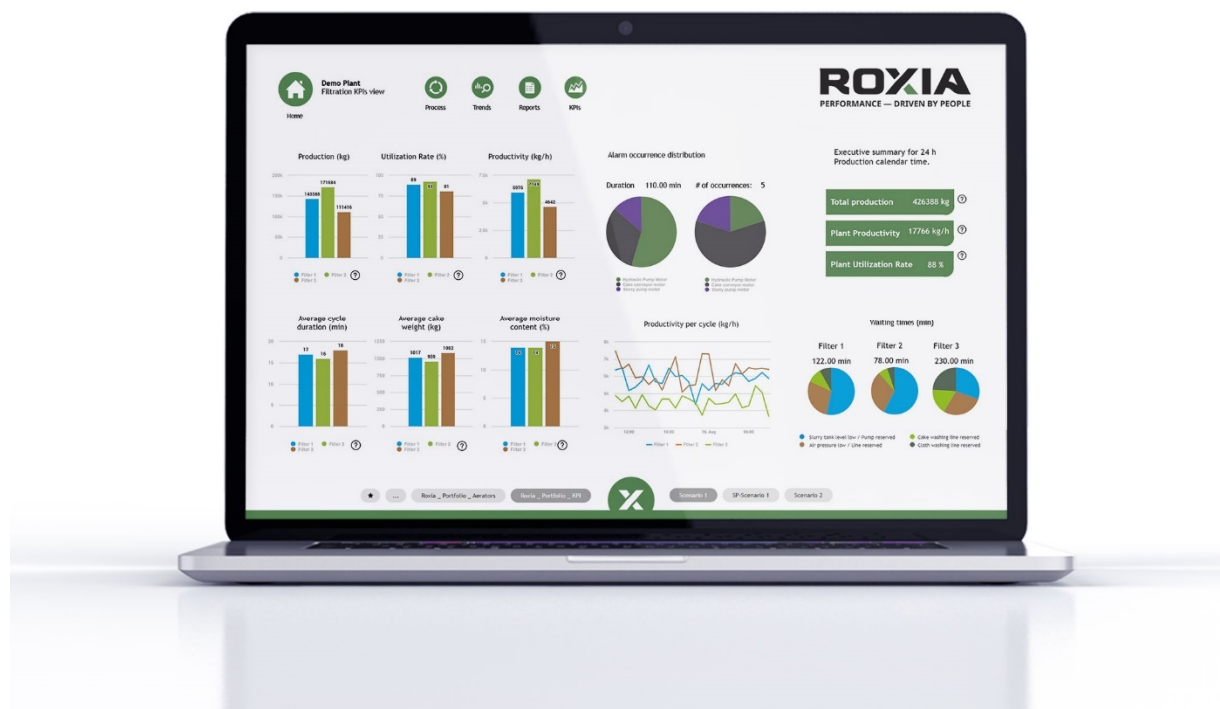
Image 1: Roxia Malibu™ is a combination of online process monitoring, maintenance, reporting and analysis tool (source: Roxia Oy)
