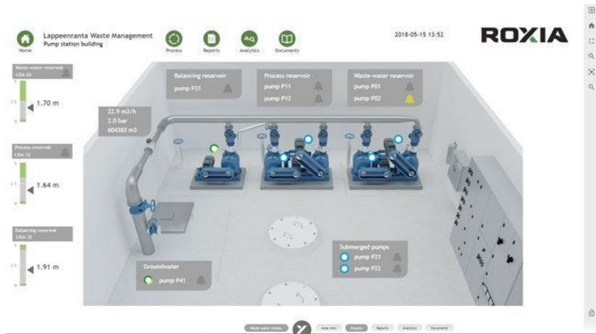
Image 3: Realistic 3D modeled environment of the filtration process (source: Roxia Oy)
