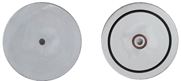
Fig.5: Die-cast test specimen made from aluminum alloy AlSi12 (Fe) with AntiCorr® coating (after 720-hour salt-spray test as per DIN ISO 9227)
