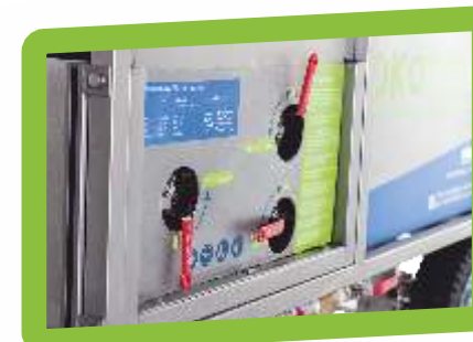
Switch between: · Return to the tank · Surface vehicle · Hose reel
