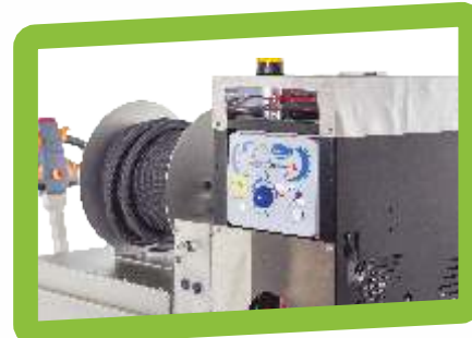
90 kW fuel oil fired burner chamber with temperature pre-selection and fault indication
