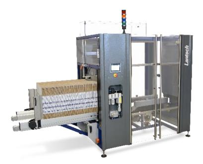
The CI-1000 case erector produces rectangular packaging fast and efficiently (© Lantech)
