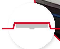
Profile membrane keypads Height: approx. 1.0 - 1.5 mm*
