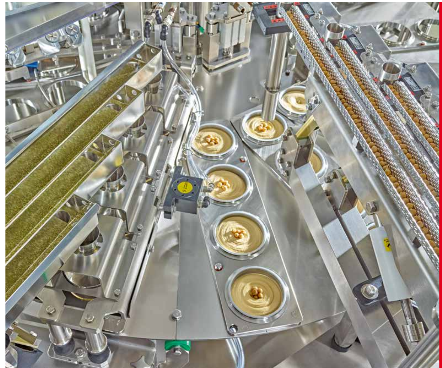
Rotary table with 4-lane ROTARY 20.000 during the filling and topping of hummus
