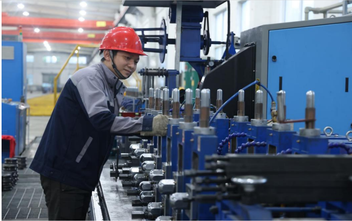
One produce lines for galvanized tube, production speed 60m/min
