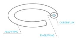
Flux cored rings are available in **silver base alloy**, **aluminum-silicon** and **aluminum-zinc** alloys.
