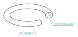
The sintered rings are indicated for **aluminum brazing** because of their homogeneous melting and better wetting. This solution avoids the poor penetration of the filler material inside the joint, typical of these applications.
