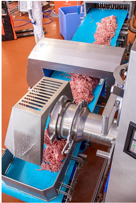
IMG_7854: The tensioning device for the pre-cutter significantly reduces the pressure on the cutting set – for a longer cutting set service life, reduced grinding cycles and a first-class cutting pattern every time.
