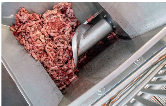
IMG_7843 and IMG_7860: The peeling edge of the feeder worm pre-cuts frozen and – as shown in this photo – ingredients containing bone, without squeezing them. At the same time, it gently conveys the material towards the meat worm by means of variably adjustable speeds. This results in a first-class cutting pattern.
