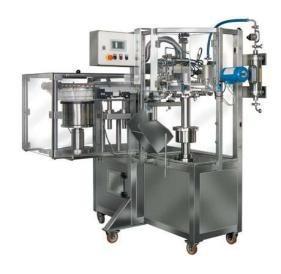
Pressure testing of the infusion bags and optional pre-processing with inert gas
