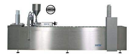
An up-to 12-track linear indexing system allows more gentle container transport
