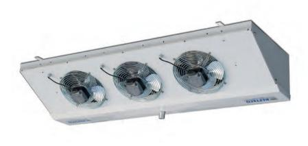
Angled air coolers super compact for small storage cold rooms with volume from 10 to 50 m3. Thanks their heavy metal construction they are suitable for storage of fresh or frozen food with temperature from -25 to +20°C.
