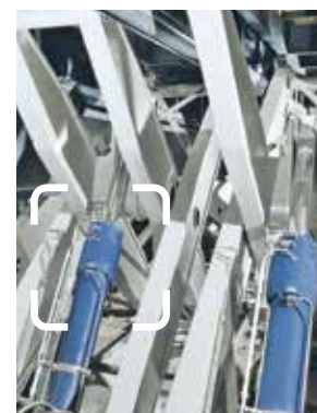
Elevating podium in a theater Stepless holding of the podium position
