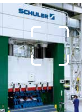
Hydraulic press Safety Catcher as mechanical restraint device, DGUV certified acc. to ISO 16902
