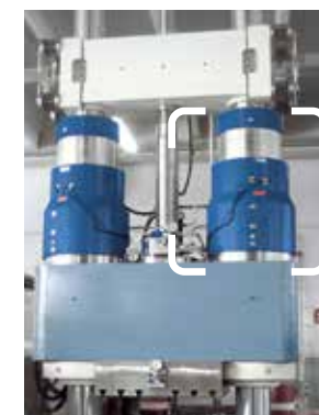
Hydroforming press Generating 400 metric tons closing force
