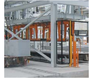
Cube Clamp STAZ with Gripper Length of 6 m
