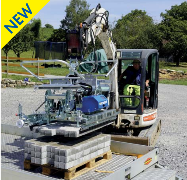
HVZ-PAVERTRON Electro-hydraulic installation clamp
