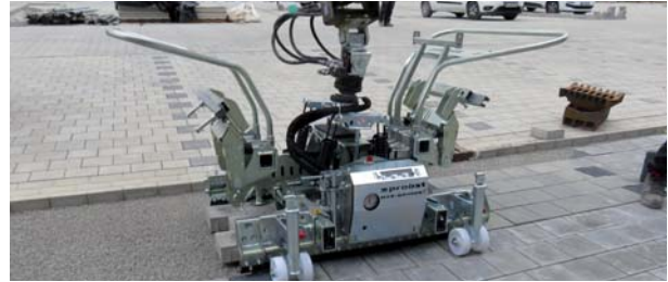
HVZ-GENIUS-II Hydraulic Installation Clamp for universal use with excavators
