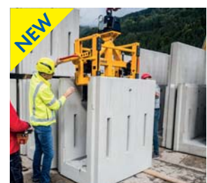
Mechanical gripper for moving trench wall elements
