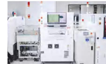
Automatic Solder Paste Inspection Machine (3D SPI)
