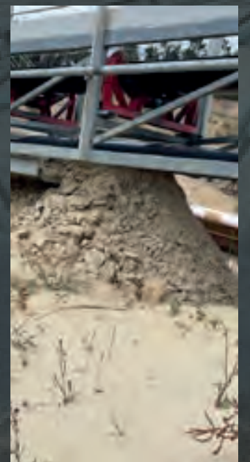
Material falling from soiled idler pulleys
