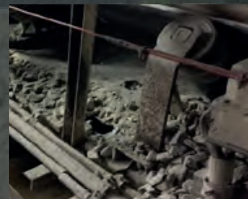
Soiling caused by poorly sealed transfer points
