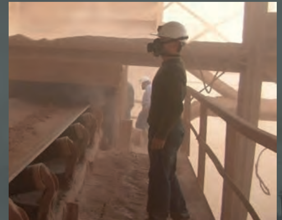
Heavy dust accumulation; full enclosure required
