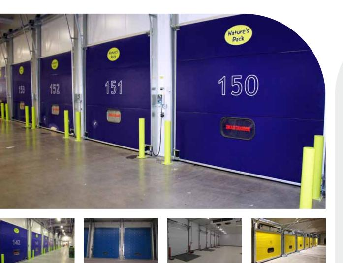
Suited for cold storage rooms, temperaturecontrolled areas. Extremely user-friendly and suitable for frequent use. The door consists of sections and is 80 mm thick. The insulation core consists of CFC-free solid polyurethane foam. The interior and exterior sheet, consisting of 0.5 mm thick galvanised steel sheet, have an oven-hardened, polyester coating. A partition between the interior and exterior sheet
