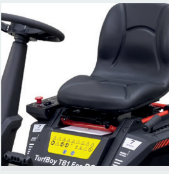
SEAT Suspended and adjustable driver seat.
