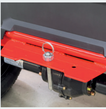
HITCH For drag matts, triangle brushes and magnet bars.
