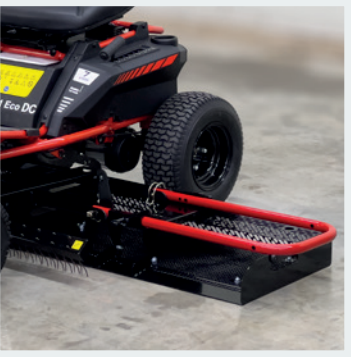
LEAVESWEEP LS900 Two optional LeaveSweeps for collecting leaves and debris with adjustable sieve from 4 – 10 mm.
