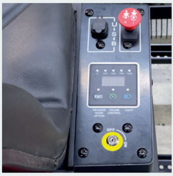
DISPLAY To control functions and battery level.
