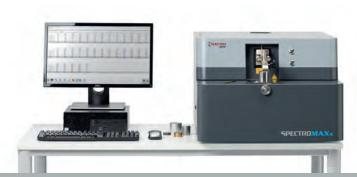
SPECTROMAXx Advanced utilizes the same high-resolution CMOS technology, with the air optic covering the same wavelengths as the basic model, from 233 nm to 670 nm. But an added UV optic handles a lower spectral range, from 120 nm to 235 nm. This includes a new capability to analyze oxygen (O) in copper. And again, a new option analyzes relevant wavelengths to 766 nm, covering potassium.
