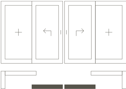
Scheme C 2 sliding sashes 2 fixed glazings sliding left + right
