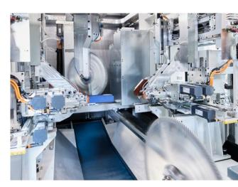
Vertical and horizontal sawing units for complex cutting, notching and combinations
