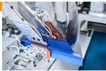
2 separate servo vertical clamps for optimum clamping
