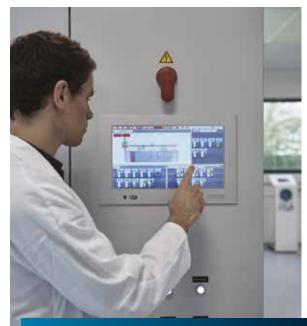
The machine controller unit allows you to setthe parameters on FISA machines. It also centralizes data and allows you to program and plan different interventions.
