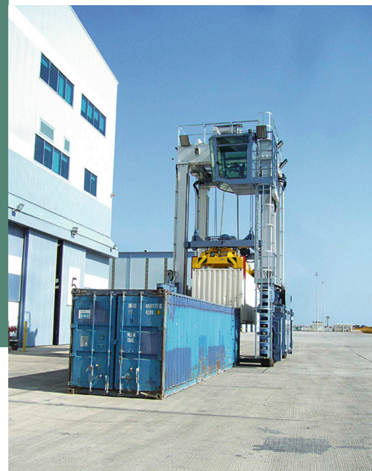
MOBILE STRADDLE TRANSPORTER Capacity: 40 t - QATAR Mobile straddle transporter for container handling
