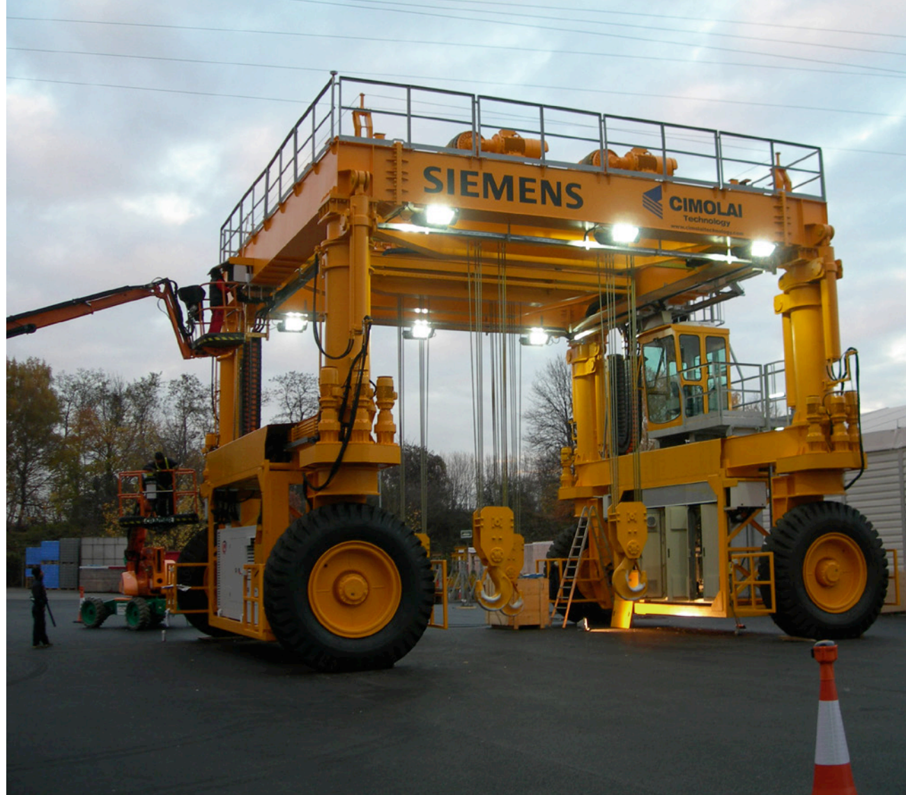
MOBILE STRADDLE TRANSPORTER Capacity: 140 t - GERMANY Special Mobile straddle transporter with adjustable dimensions
