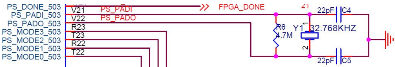
Figure 2-6-2: Passive Crystal Oscillator for RTC
