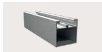
P 9522 Aluminium profile Partial support fixed installation or total support floating installation Max. support distance 500 mm 50x50 mm
