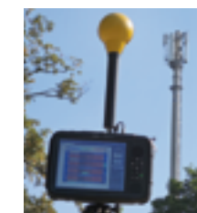
SignalShark connected to Three-Axis-Antenna (200 MHz - 8 GHz)
