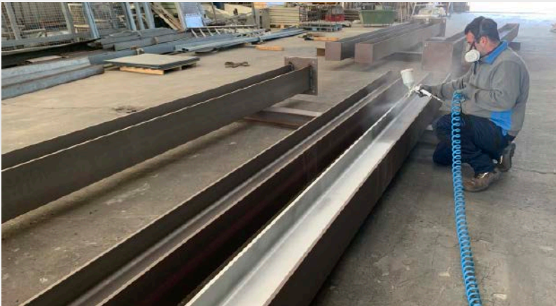
Example of application of Tecnadis Multicoat Anticorrosion (Primer) on a slightly oxidised surface
