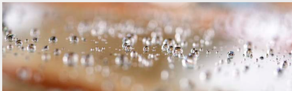
Example of the hydrophobic effect of TECNADIS GWR on a car windscreen.
