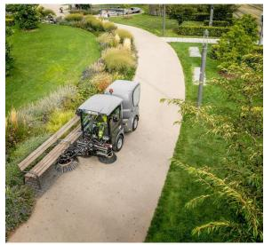
The flow-optimised suction system delivers excellent results, even at low engine speed, and is very fuel-efficient. The cleaning performance is comparable to that of the superior 2  $m^3$  model class.
