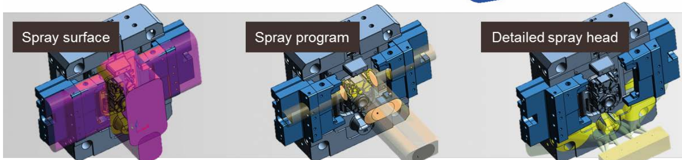
Simulation of the spraying process in different levels of detail adapted to the casting and tooling development phase
