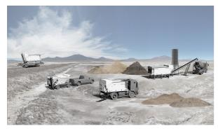
Another Blend product which has a high market demand is the E-series range of mobile plants. Thanks to the internal structure which stocks raw materials in separate compartments, there is no waste of material and only the necessary is mixed in small or large quantities, directly on-site, enabling you to obtain a fresh and high-quality product, with no additional transport, saving time and costs. By changing the recipe it is possible to mix different qualities of concrete with the same load.
