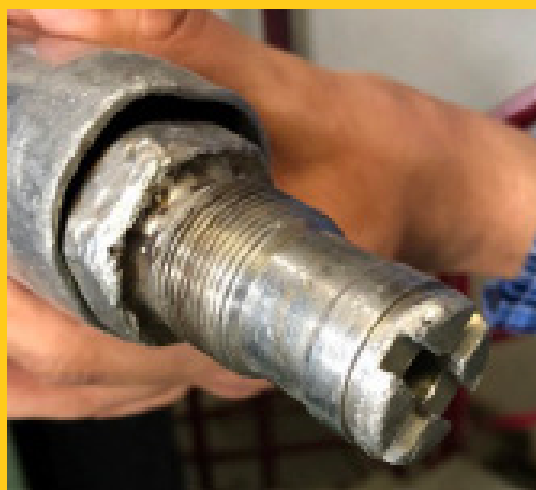
Damage to threads on SDX 3 Nozzle
